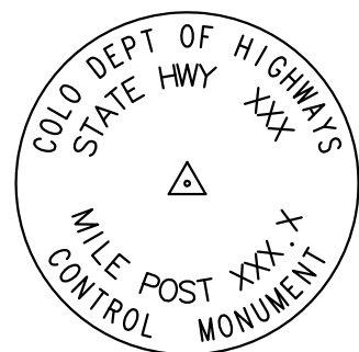
Typical Control Monument Cap Not to Scale
